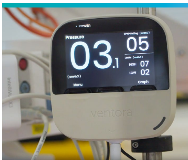
Ventora’s Airway Pressure Monitor clinical prototype, developed as part of their CTCM project.
