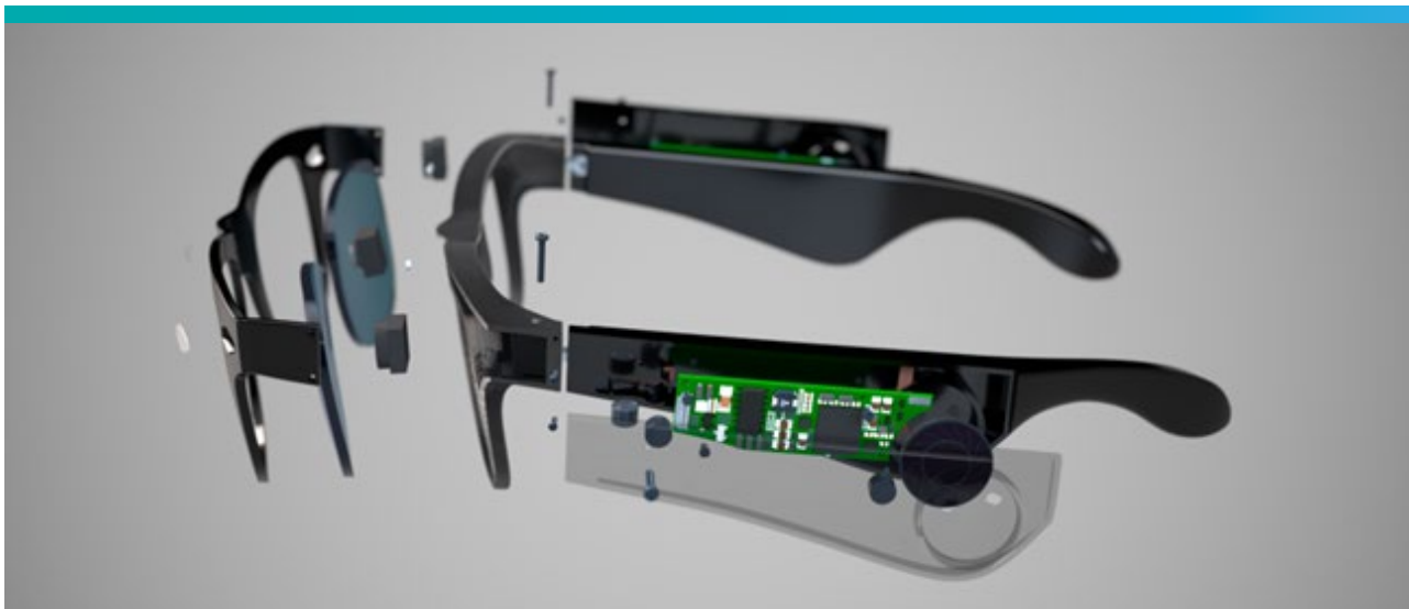
The ARIA 'Vision via Sound' glasses for blind users - exploded view of 'Hollywood' model.
